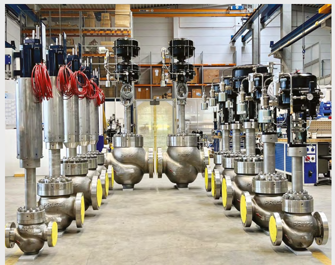
Set of fuel gas valves capable of handling 100% hydrogen
