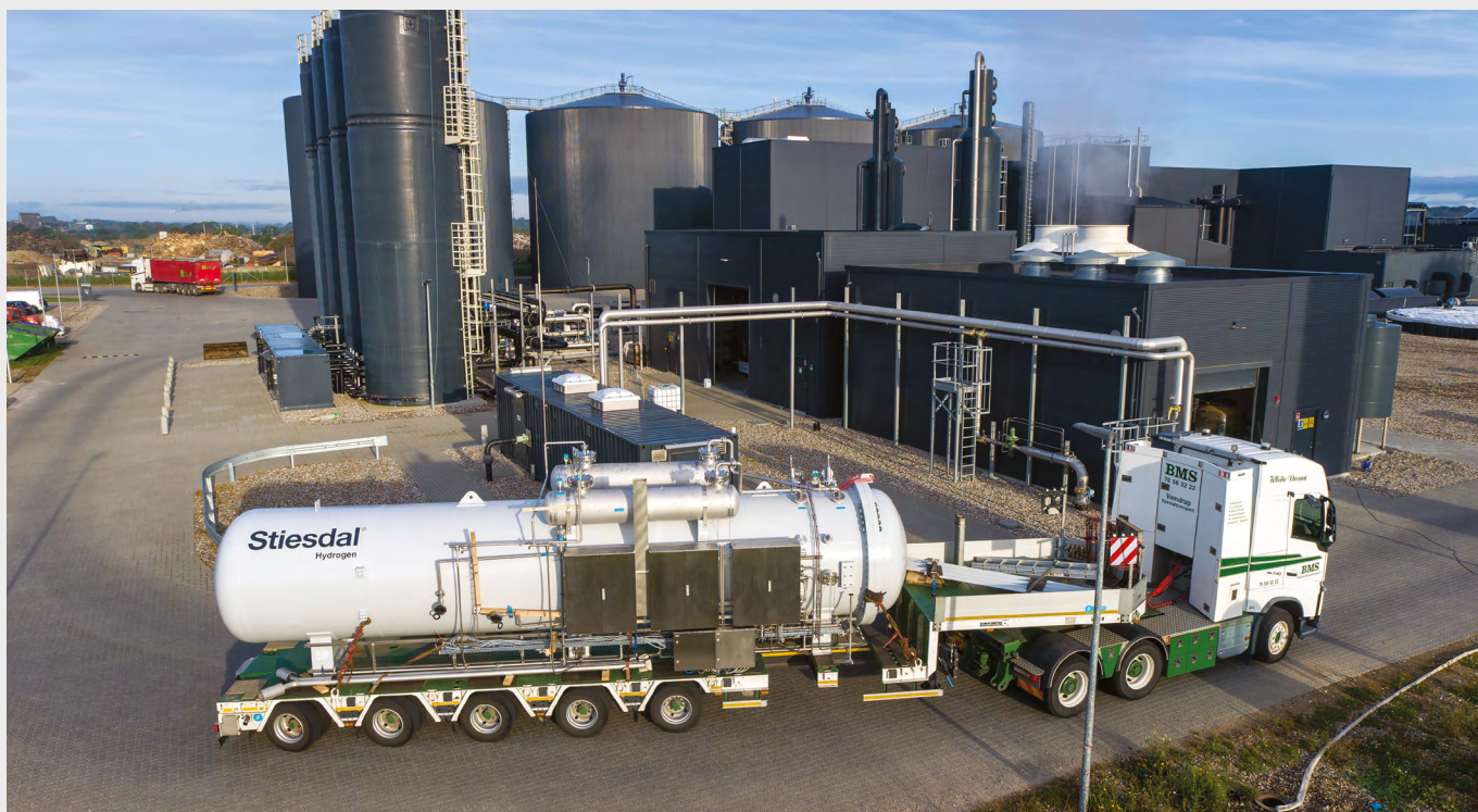
All components for the HydroGen Electrolyzer are delivered to the site on two standard trucks: one truck (above) for the main pressure vessel, and one truck for the power and auxiliary modules.
