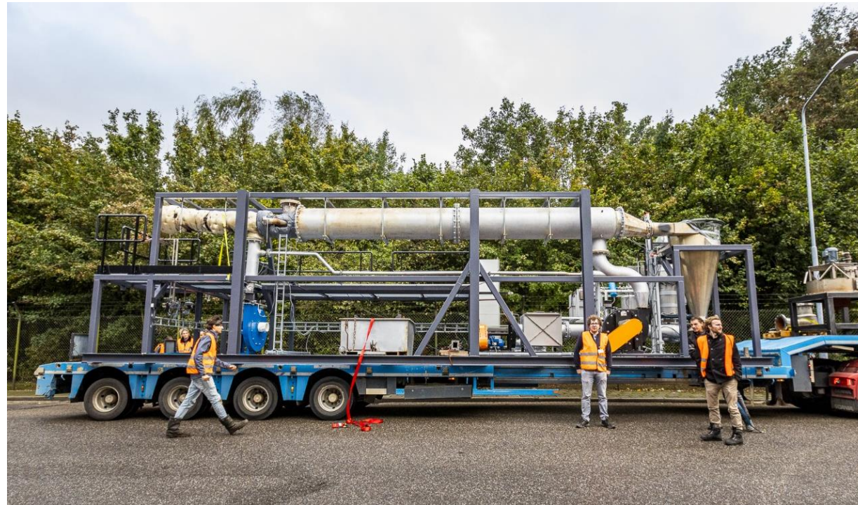
First industrial combustion pilot at Swinkels Brewery 100 kW
