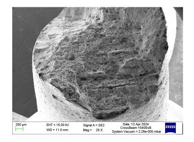
EN 1.4435 – 13% Ni Dimples, ductile fracture
