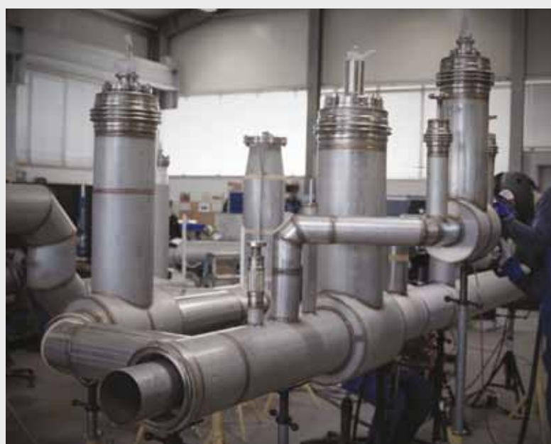
BUTTING CryoTech's vacuum insulated piping (VIP) valve skid
