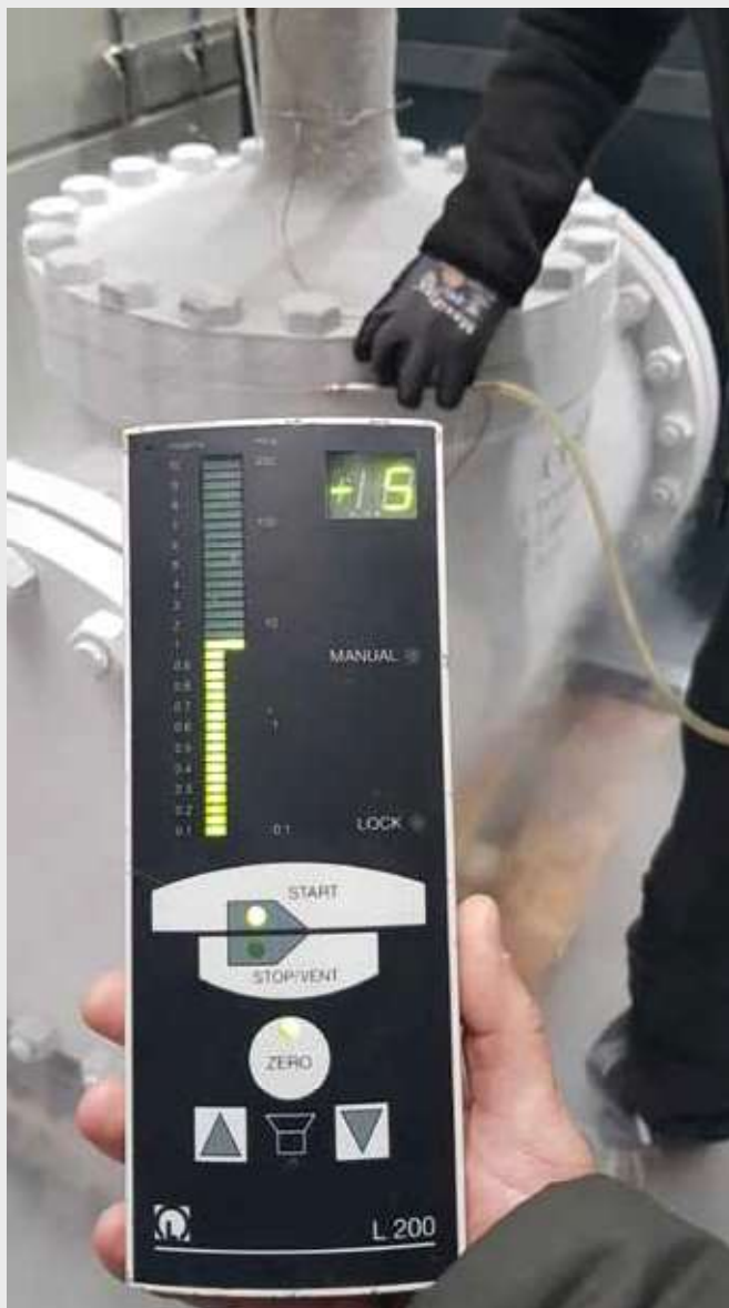
Fugitive emission test with a DN 500 Quadax® top entry butterfly valve
